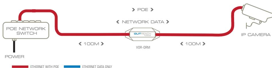
Diagram 1. A single OUTREACH Max doubles the cable range to a POE IP Camera. Each cable segment can be up to 100 metres.
