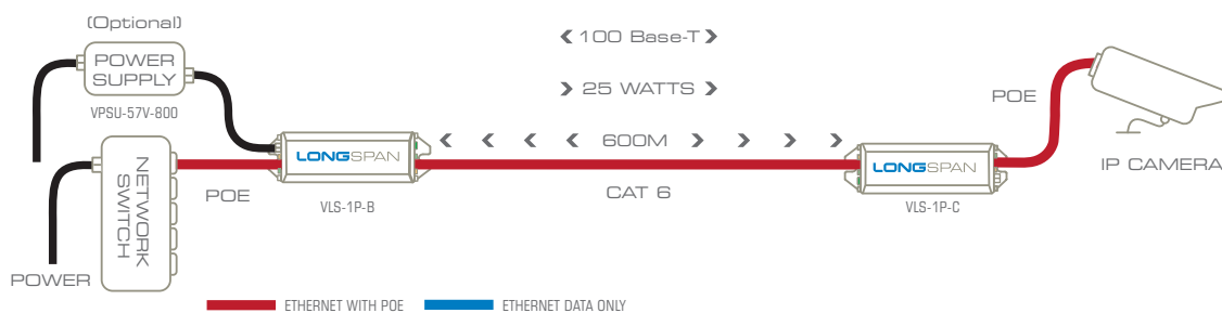
Diagram 1. A pair of LONGSPAN converters deliver full-bandwidth Ethernet & optional full-power POE over greatly extended distances of regular network cable or UTP.
